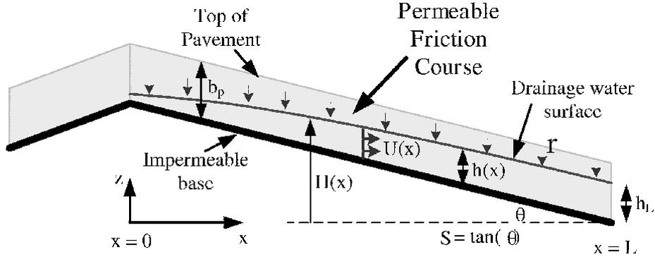
Figure 1: Schematic view of drainage in a porous layer (adapted from *Charbeneau and Barrett* (2008), with permission of AGU)
