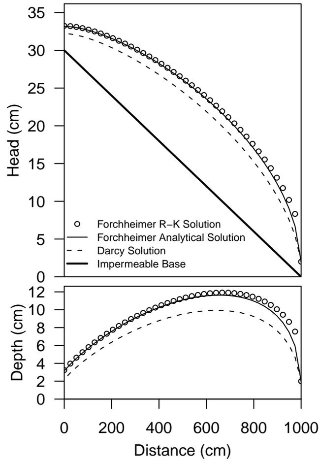
Figure 4: Comparison of drainage profiles computed using Forchheimer's equation and Darcy's law for rainfall at 5cm/hr, slope of -3%, hydraulic conductivity 3 cm/s, and  $\beta = 0.64s^2/cm^2$ , and  $h_L = 2cm$ . R-K refers to 4th order Runge-Kutta integration using 40 steps.
