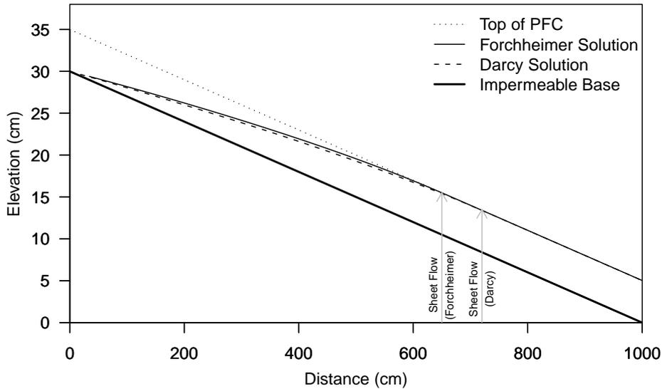
Figure 5: Drainage profiles for a 5cm porous layer with sheet flow under Forchheimer (solid) and Darcy (dashed) flow. Parameters were  $K = 2\text{cm/s}$ ,  $\beta = 0.984\text{s}^2/\text{cm}^2$  by power fit, and rainfall of 1.5 cm/hr.
