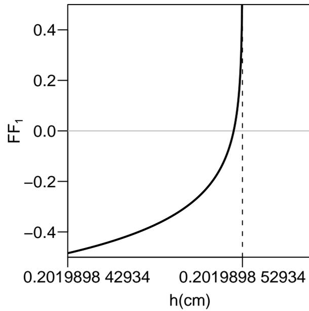
Figure 3: Variation in the implicit solution function for Case 1 (low rainfall rates) when  $x = 50\text{cm}$  and other parameters are the same as Fig. 2. The root lies  $5.0277 \cdot 10^{-10}\text{cm}$  from the asymptote.
