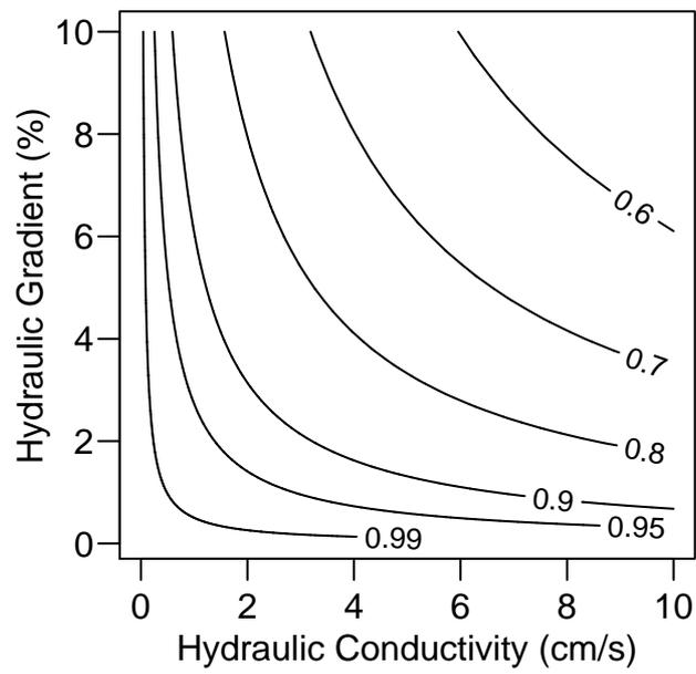
Figure 8: Contours of the discharge ratio ( $\Phi = q_{Forchheimer}/q_{Darcy}$ ) as a function of hydraulic conductivity and hydraulic gradient for porous asphalt overlays. The Forchheimer coefficient and hydraulic conductivity have been related by Eq. 42.
