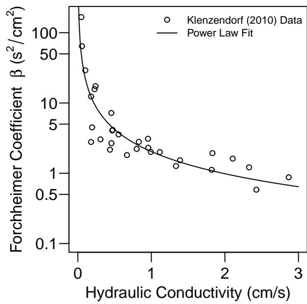
Figure 6: Comparison of Forchheimer coefficient and hydraulic conductivity for permeable friction course in the results of Klenzendorf (2010).
