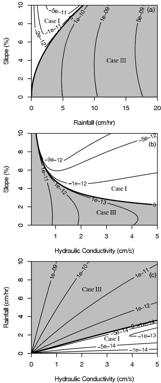
Figure 7: Contours of the discriminant (Eq. 13) for (a) hydraulic conductivity held constant at 1 cm/s; (b) rainfall held constant at 2cm/hr; and, (c) slope held constant at -3%. The discriminant is positive in areas shaded gray (Case III) and negative in white areas (Case I). The hydraulic conductivity and Forchheimer coefficient are related using Eq. 42.
