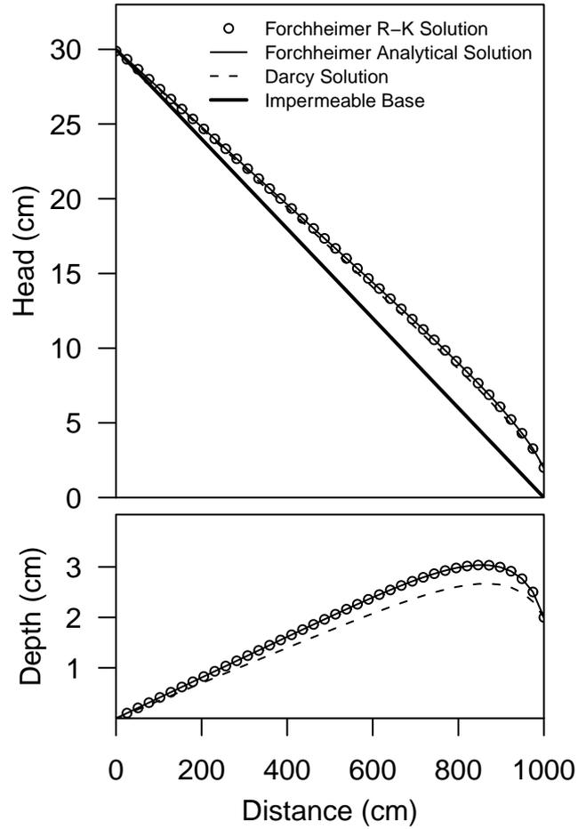
Figure 2: Comparison of drainage profiles computed using Forchheimer's equation and Darcy's law for rainfall at 1cm/hr, slope of -3%, hydraulic conductivity 3 cm/s,  $\beta = 0.64s^2/cm^2$ , and  $h_L = 2cm$ . R-K refers to 4th order Runge-Kutta integration using 40 steps. Discriminant is negative for this case as shown in Fig. 7(c).
