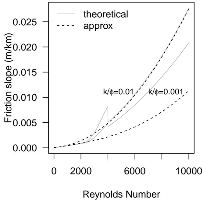
Figure 1. Smoothed model compared to theoretical values at lower Reynolds numbers. Slope at zero is found from laminar conditions.
