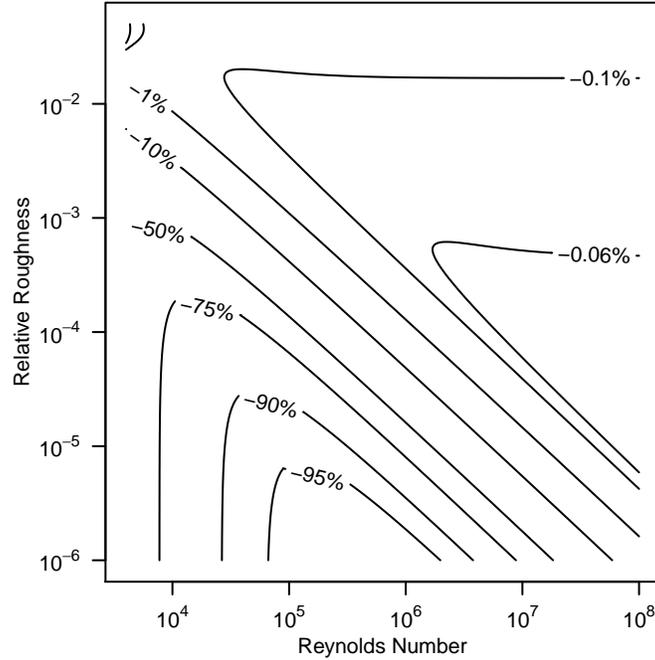
**Figure 3. Relative errors of smoothed approximation with Hagen-Poiseuille slope at zero flow considering water at 20C.**
