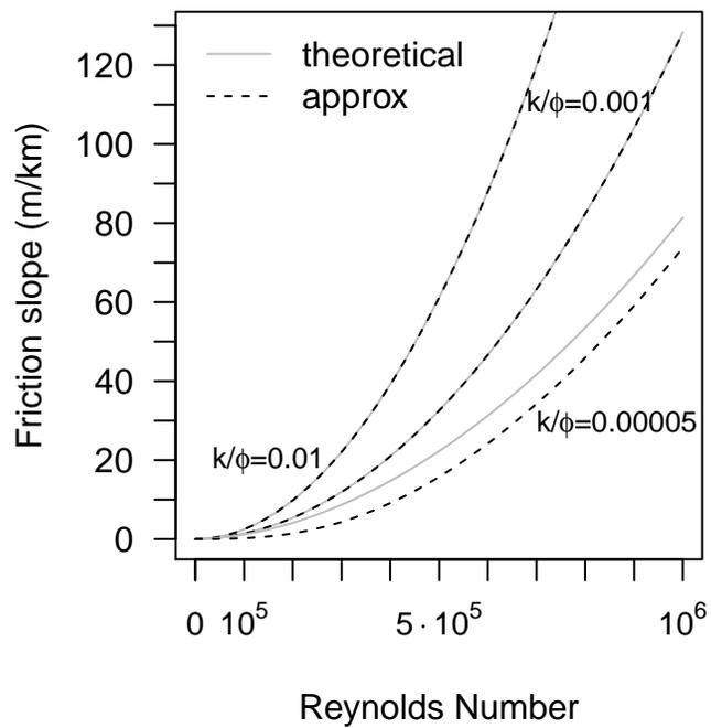
Figure 2. Smoothed model compared to theoretical values at higher Reynolds numbers. Slope at zero is found from laminar conditions.
